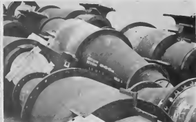
NEW CYCLONES will be installed in the PCAR Cat Cracker next spring. The cyclones will be hung upright in the reactor to separate the catalyst from the vapors. Dust pots are secured below them, with dipsles extending downward into the catalytic ages.
